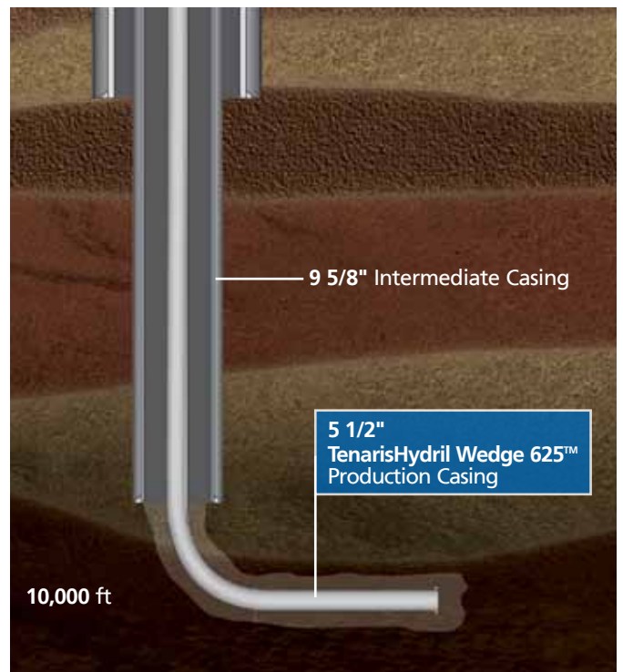
▲ TenarisHydril Wedge 625™ connections in the Granite Wash shale horizontal well.
